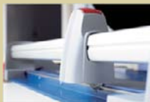
Circular blade in plastic head
